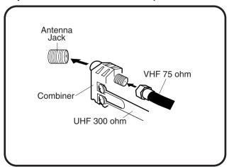
Connect the VHF 75 ohm cable and UHF 300 ohm Twin-lead Wire to the Combiner. Attach the Combiner to the Antenna Jack.
